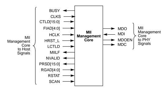
Figure 2.3 MIIM Core Interface Diagram
