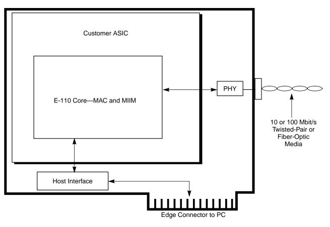
Figure 1.5 Network Interface Card Block Diagram
