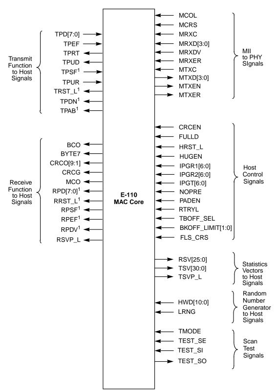
Figure 2.1 E-110 MAC Core Interface Diagram
