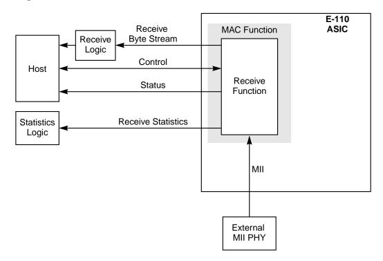
Figure 3.8 Receive Function Interface
